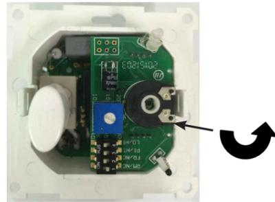
**Tip:** When installing the temperature setting dial, make sure the potentiometer is turned clockwise as far as possible. The dial will then "snap on" at 9.
