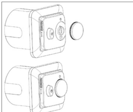
Attach the temperature setting dial and finish the installation.
