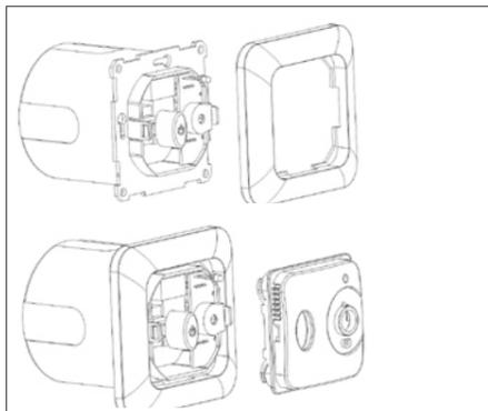
Install the frame and the thermostat housing.
