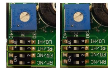
DIP-switch 3 is in the left position (HT/Heating)
