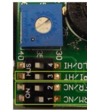
DIP-switch 3 is in the left position (HT/Heating)
