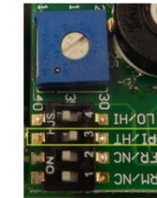
DIP-switch 3 is in the right position. DIP-switch 4 is in the position according to the load of the thermostat as described under point 1. Other DIP-switch positions are not important.
