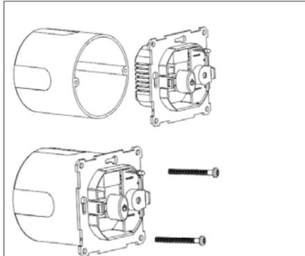
Connect wires (power supply, heating cable and sensor cable (if relevant), and install the thermostat in the junction box.
