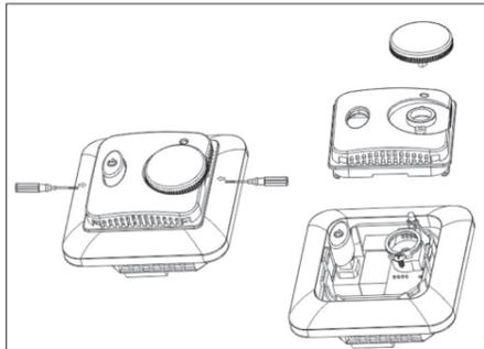
Remove the dial and release the housing by pressing on the spring clips on both sides, using e.g. a small screw driver.
