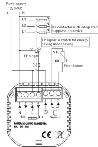
NOTE: The maximum relay load of the thermostat is 16A. However, in order to secure an optimal life time of the thermostat, a maximum load of 14A is recommended. A higher load will shorten the lifetime of the electrical components.
