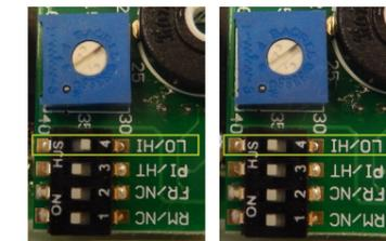
LO: DIP-switch is in the right position when the load is less than 10A
